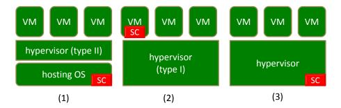
Fig. 6. Possible placement of the attestation supporting component.
