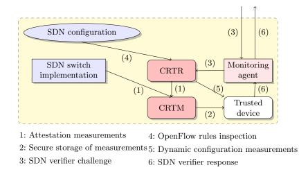
Fig. 3. Network element component architecture target
