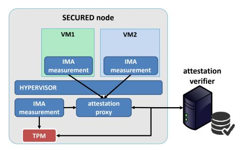
Fig. 7. IMA-based attestation architecture.
