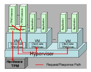
Fig. 4. The vTPM architecture [10].
