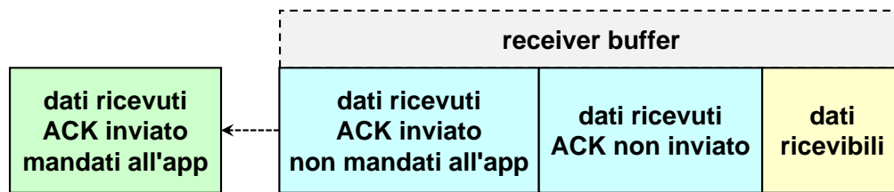
Figura 2.11: TCP: sliding window
